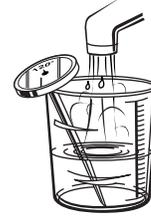
3. Check the temperature on the thermometer as the water is running into the cup.
