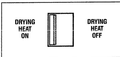
**DRYING HEAT ON.** Turns the drying heater on for fast drying.
