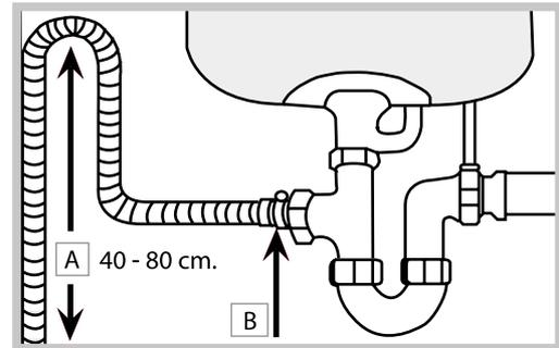
The outlet hose must be at a height ranging from 40 to 80 cm (from 15" to 31") from the floor / surface where the dishwasher rests (A).
