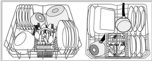
Several dishwasher models are fitted with tip-up sections\*, which can be used in a vertical position when arranging plates or in a horizontal position when arranging saucepans, salad bowls and frying pans.
