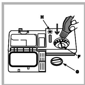
1. Open the dispenser by turning the lid (G) in an anticlockwise direction.
