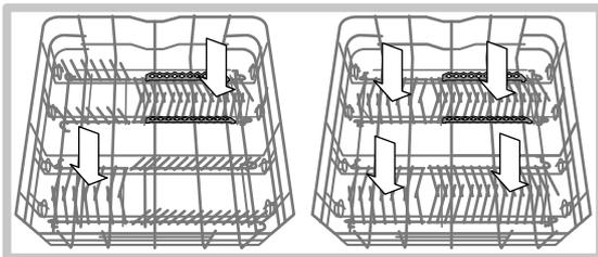
The type of cutlery basket may vary (modular or non-modular) according to the dishwasher model. The non-modular basket must **only** be positioned at the front of the lower rack.
