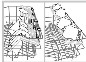
The tip-up compartments can be positioned at different heights, to optimise the arrangement of crockery throughout the rack. Wine glasses can be placed safely in the tip-up compartments, by inserting the stem of each glass into the
