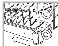
Open the left and right guide rail stops and pull out the rack; position it higher or lower as required, slide it along the guide rails until the front wheels are in place and close the stops (*see figure*).
