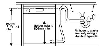
NOTE: Ensure the sink outlet pipe has a minimum diameter of 32mm.
