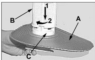
Reassemble the filter parts (as shown in the figure) and reinsert the whole assembly into the dishwasher. Position it into its housing and press downwards. The dishwasher is not to be used without filters. Improper replacement of the filters may reduce the efficiency of the wash and even damage your dishwasher.
