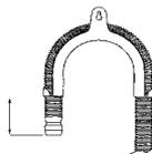
**DO NOT** position the standpipe near an electrical outlet. **ENSURE** that the drain hose is not kinked and it is routed as shown in the diagram.
