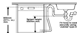
**NOTE:** Ensure the sink outlet pipe has a minimum diameter of 32mm.
