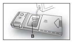
After pouring the detergent into the container, close the lid, firstly pushing (1) and then pressing on it (2) until you hear the click.
