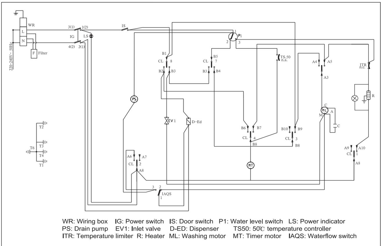
WR: Wiring box IG: Power switch IS: Door switch P1: Water level switch LS: Power indicator
