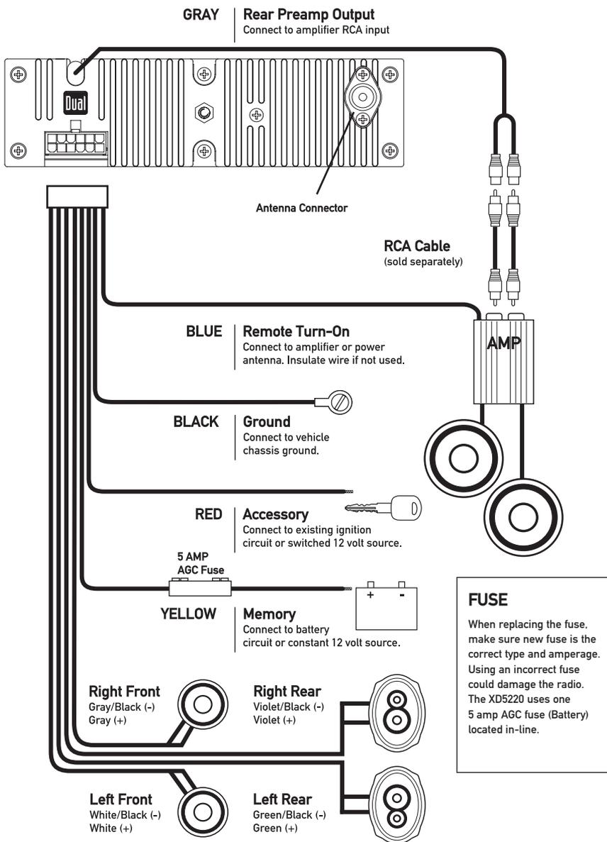
\* CAUTION - Do not attach any speaker leads to ground as severe damage will occur.
