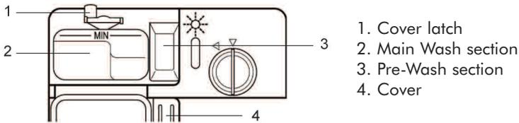
The larger Main wash section automatically empties detergent into the dishwasher during the wash ( See the "cycle Selection Charts" )
