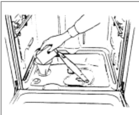
**The salt container must be filled when the "low salt" indicator light (located on the control panel) comes on.**
