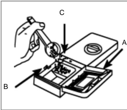
**Note:** To facilitate closing the cover, remove any excess detergent on the edges of the dispenser.
