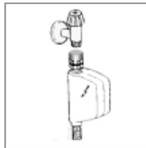
After turning off the water tap, unscrew the end of the water supply hose, remove the filter and clean it carefully under running water. Then, return the filter to its place and tighten the water supply hose back into position.
