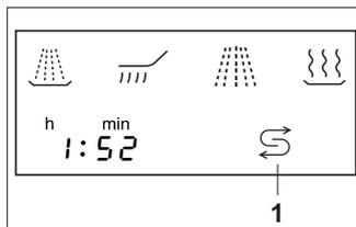
The salt container must be filled when the "low salt indicator" (located on the control panel) lights.
