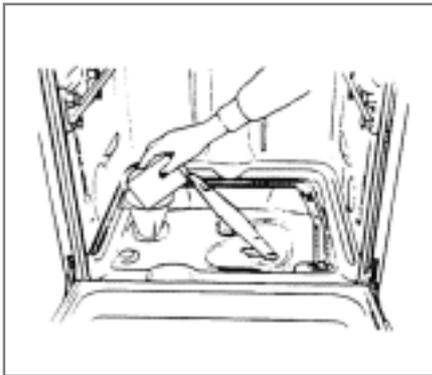
The salt container should be filled after about every 30 wash cycles.
