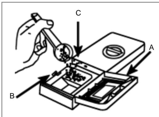
**Notice:** To facilitate closing the cover, remove any excess detergent on the edges of the dispenser.
