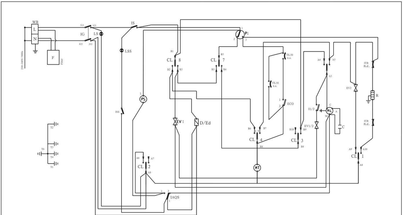
WR: Wiring box IG: Power switch IS: Door switch P1: Water level switch LS: Power indicator LSS: Salt missing switch
