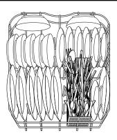
When loading the lower rack, do not load large platters or trays in the front left corner. They may prevent detergent from circulating during the wash cycle.
