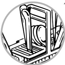
A cover can be lowered to either side to secure lightweight items from the effects of the vigorous wash action.
