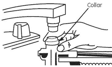
**Note:** The uncouple's small hose carries water from the faucet to the dishwasher. The large hose carries water from the dishwasher to the sink. Orient the faucet with uncouple attached so water from the uncouple will run into the sink drain.
