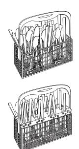
The silverware basket may be used without the topper for quick loading. With the topper, flatware is better positioned for the dishwasher to thoroughly wash and dry all pieces by preventing nesting.
