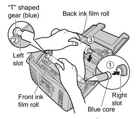
If the ink film is slack, tighten it by winding the gear.
