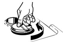
**NOTE:** To open detergent cup after it has been closed, simply turn the detergent cup handle counterclockwise until it releases. A snapping sound may be heard.
