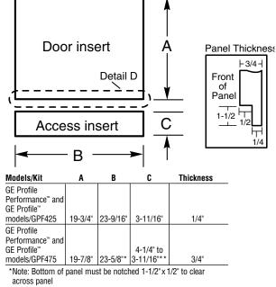
\*\*Adjustment required to match adjacent cabinets fronts due to leveling leg adjustment, 4" nominal.
