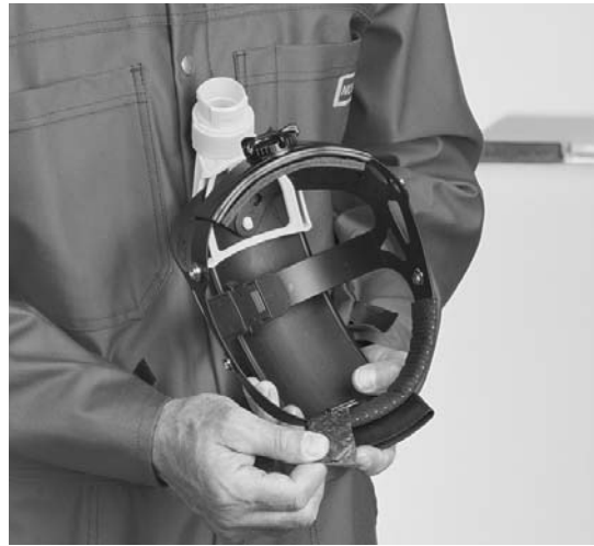
FIGURE 9 REPLACER LE BANDEAU ABSORBANT
