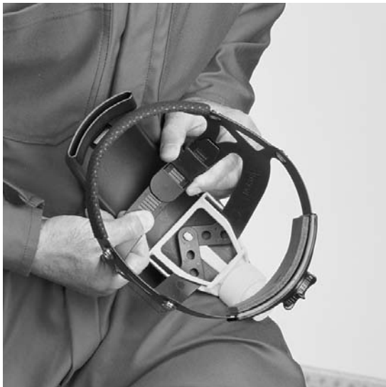
FIGURE 3 WIDEN THE CENTER LATERAL STRAP
