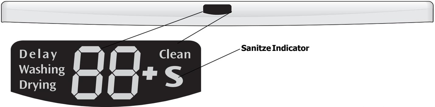
The WASHING light comes on at the beginning of cycle and remains on throughout the wash and rinse phases of the cycle.
