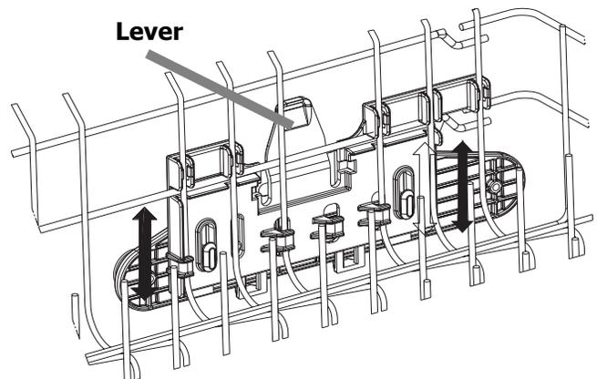
To lower the upper rack, press the lever and push down on the rack.
