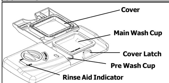
**If the cover is closed on the Main Wash Cup, open by pressing the cover latch.**
