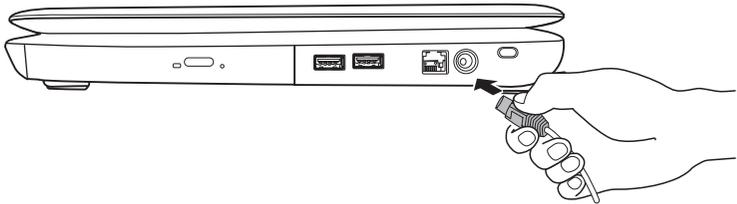
*Figure 3-3 Connecting the adaptor to the computer*
