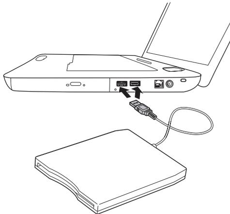
*Figure 8-7 Connecting the USB floppy diskette drive*
