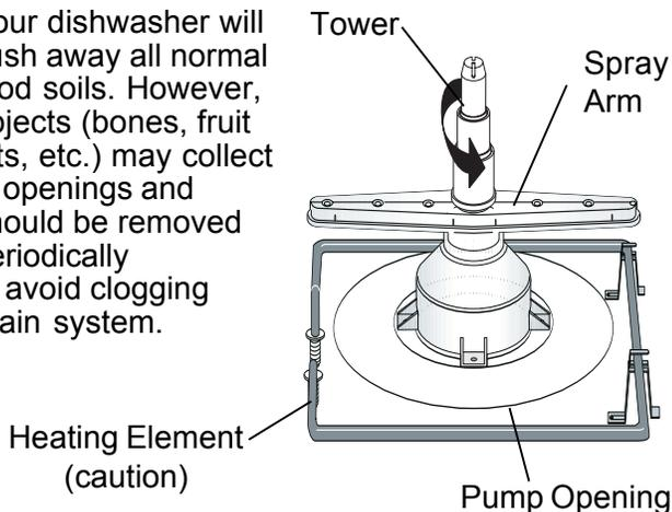
1. Remove tower base by turning counterclockwise.
