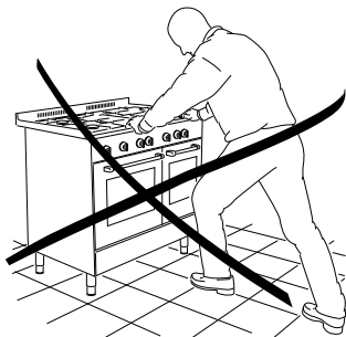
Figure 7 Incorrectly moving the cooker
