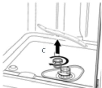
Fig. 12 Removing the spray arms (C and D)
