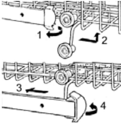
Fig. 5 Adjusting the upper rack for model DW60CSW1/DW60CSX1
