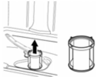
Fig. 11 Removing the filter unit (Filter B)
