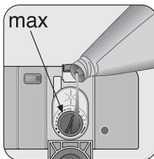
Fill up with rinse aid. The maximum level for filling is indicated by "max"
