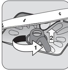
Turn the handle about 1/4 turn anticlockwise and remove filters **B** and **C**.
