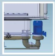
Self-draining wash pumps provide maximum hygiene with no smells and all wash and rinse zones drain automatically at the push of a button.
