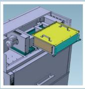
Different components, such as the energy saving device and all the washing and rinsing arms are easily removable from their housing for cleaning.
