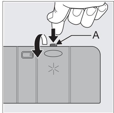
2. Add the rinse aid in the container. The maximum level for filling is indicated by "max".
