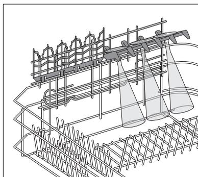
1. Remove beer glass holders by pulling upwards and pressing lightly on the hooks from below.
