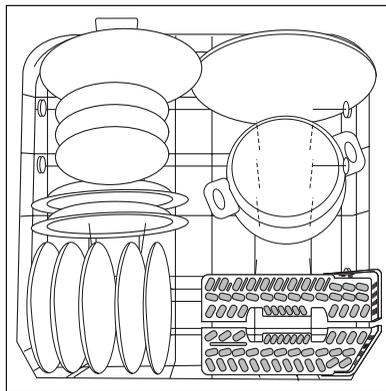
To make it easier to load larger dishes, all rear plate racks in the lower basket can be folded down.
