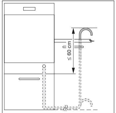
The total length of the drain hose, including any extension you might add, must be no longer than 4 metres. The internal diameter of the extension hose must be no smaller than the diameter of the hose provided.
