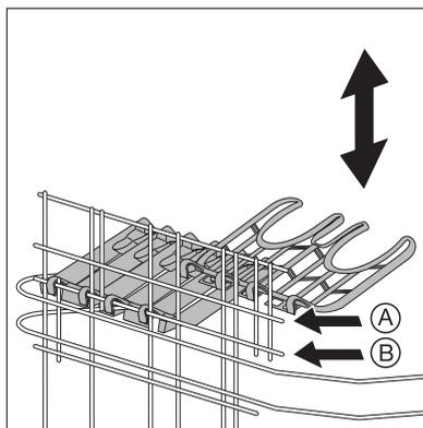
The bars that fix the beer glass holders or cup racks can be removed, if required.
