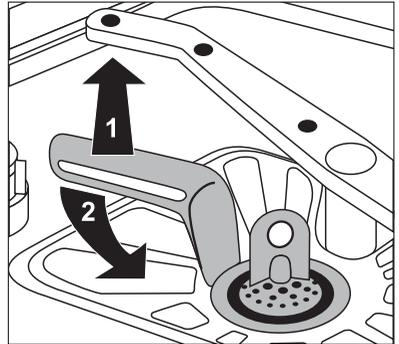
6. Remove the flat filter from the base of the washing compartment and clean both faces thoroughly.
