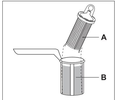
3. Turn the handle about 1/4 a turn anticlockwise and remove the filter system.
