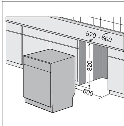
By removing the machine's worktop, you can install it under a close fitting sink unit or a pre-existing top, providing the dimensions of the recess correspond to those shown in the picture.
