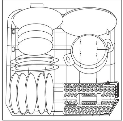
To make it easier to load larger dishes, the 2 plate racks on the right in the lower basket can be folded down.
