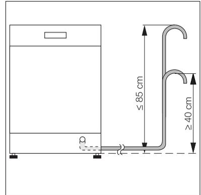
If you use a drain hose extension it must be no longer than 2 metres and its internal diameter must be no smaller than the diameter of the hose provided.
