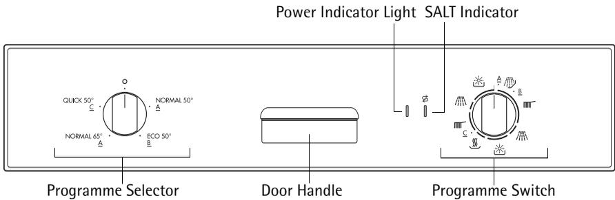
Set the point at which the wash programme is to start using the **programme selector**. The programme switch rotates during the wash programme and indicates the position that has been reached in the programme.
