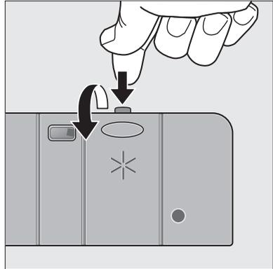
4. Fill with rinse aid exactly up to the level marked "max"; this corresponds to a quantity of approx. 140 ml.
