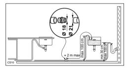
The sink plug must not be in place when the machine is draining as this could cause the water to siphon back into the machine.
