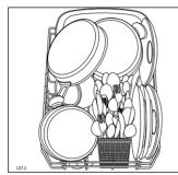
The two rear rows of prongs on the lower basket can be easily lowered to allow you to load pots, pans and bowls.
