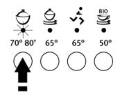
The current level is indicated by the number of flashes made by the **Intensive 70° 80'** indicator light, that alternates 5 seconds off with a number of flashes, this continues for about 60 seconds.
