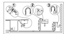
The waste connection must be at a height of between 30 cm (minimum) and 100 cm (maximum) from the bottom of the dishwasher.
