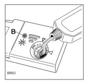
If rinse aid refilling is necessary, the rinse aid indicator light will illuminate only in setting mode and at the end of the washing programme.
