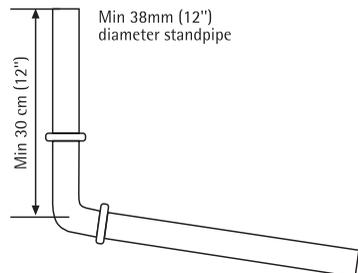
Min 38mm (1 1/2") diameter standpipe
