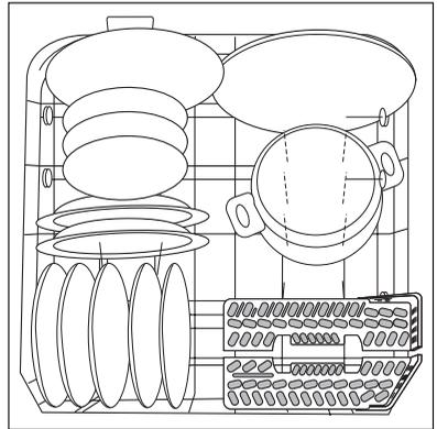
To make it easier to load larger dishes, the two plate racks on the right in the lower basket can be folded down.
