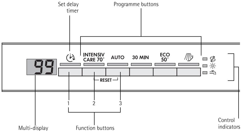
The **Programme buttons** are used to select the desired dishwashing cycle.
