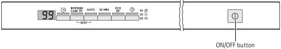
The **ON/OFF button** is used to turn the dishwasher on and off.
