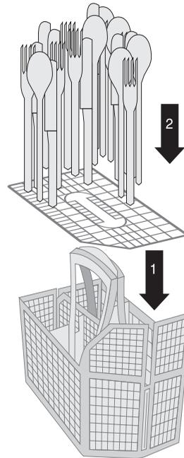
To make the removal of cutlery easier, **on some dishwasher models** it is possible to open the cutlery rack. If you use the grid insert then the cutlery rack cannot be opened.
