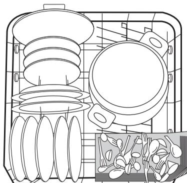
**i** To ease the loading of large items at **some dishwasher-models** the two rows of prongs for the right-hand plate insert can be folded down:
