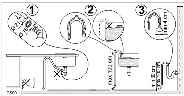
The waste connection must be at a height of between 30 cm (minimum) and 100 cm (maximum) from the floor.
