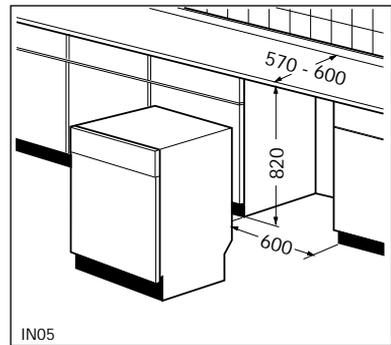
Insert the machine after adjusting height and levelling with the adjustable feet. When inserting the machine, ensure that the water inlet and drain hoses are not kinked or squashed.
