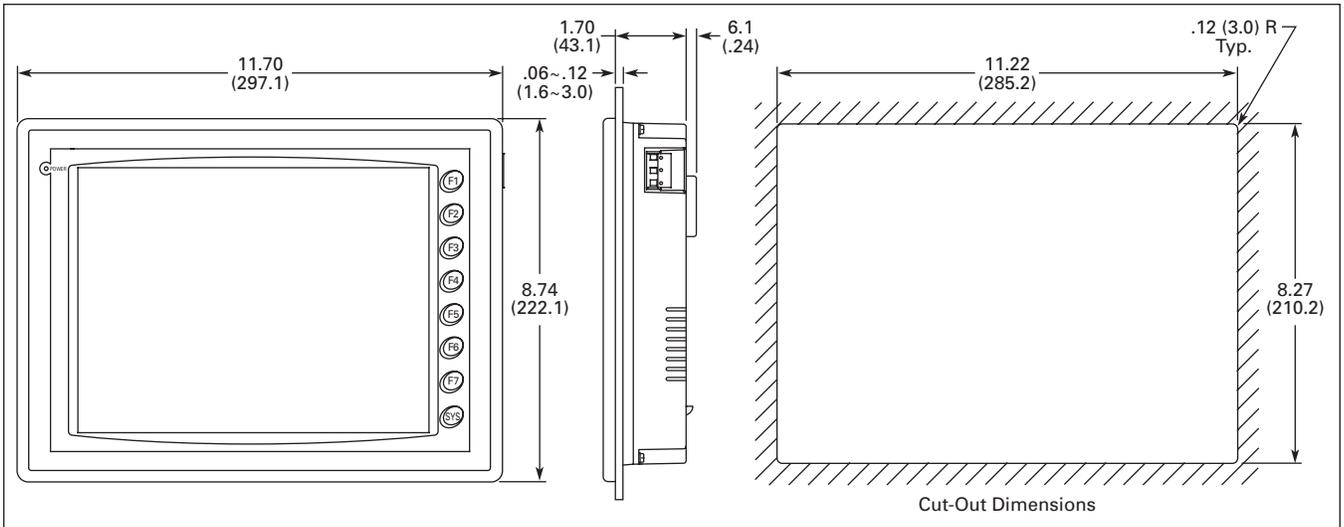
**Figure 11. HMI10CE — Approximate Dimensions in Inches (mm)**
