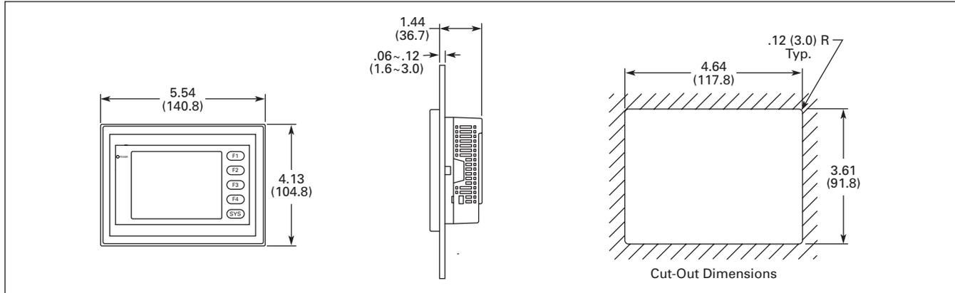
Figure 8. HMI04\_\_ — Approximate Dimensions in Inches (mm)
