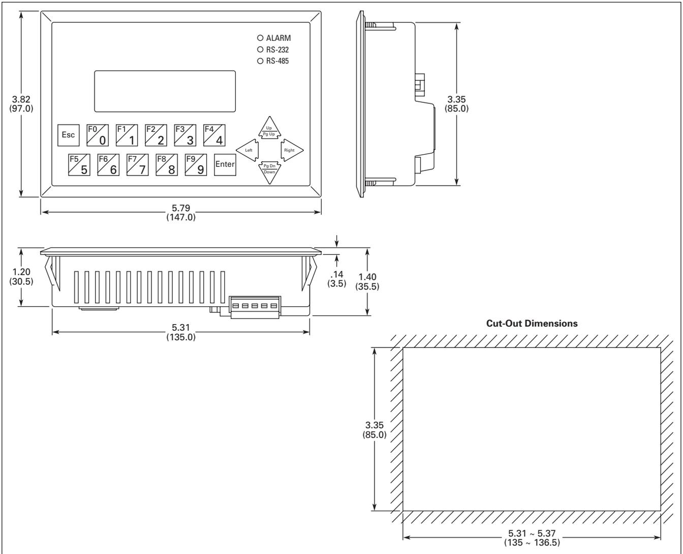
**Figure 5. ECL-GP02 — Approximate Dimensions in Inches (mm)**
