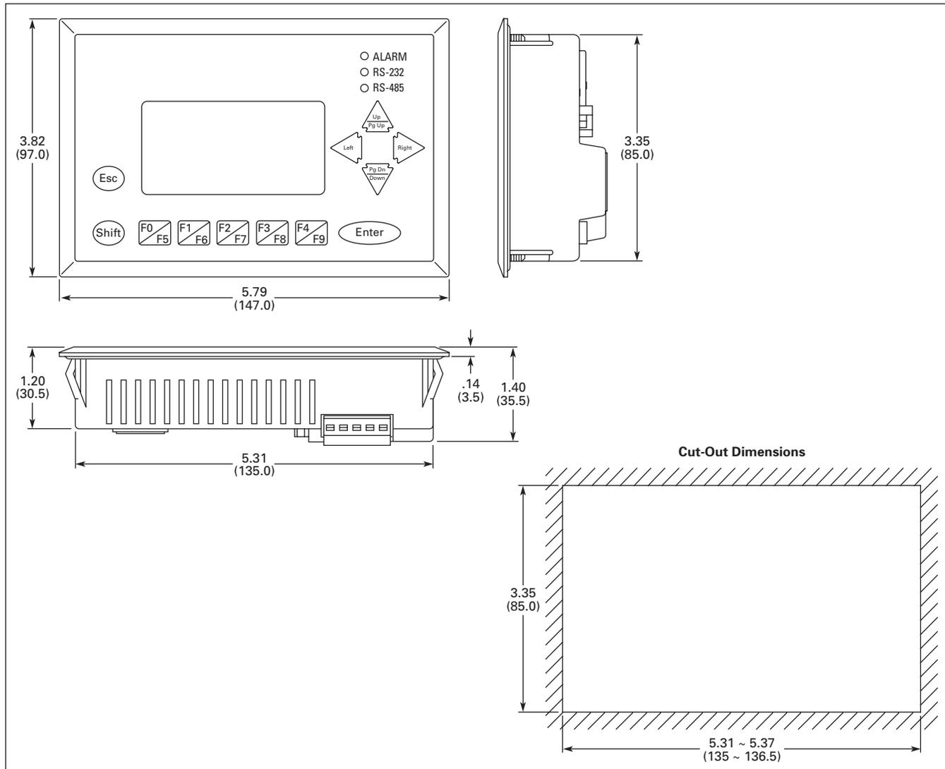
Figure 4. ECL-GP04 — Approximate Dimensions in Inches (mm)
