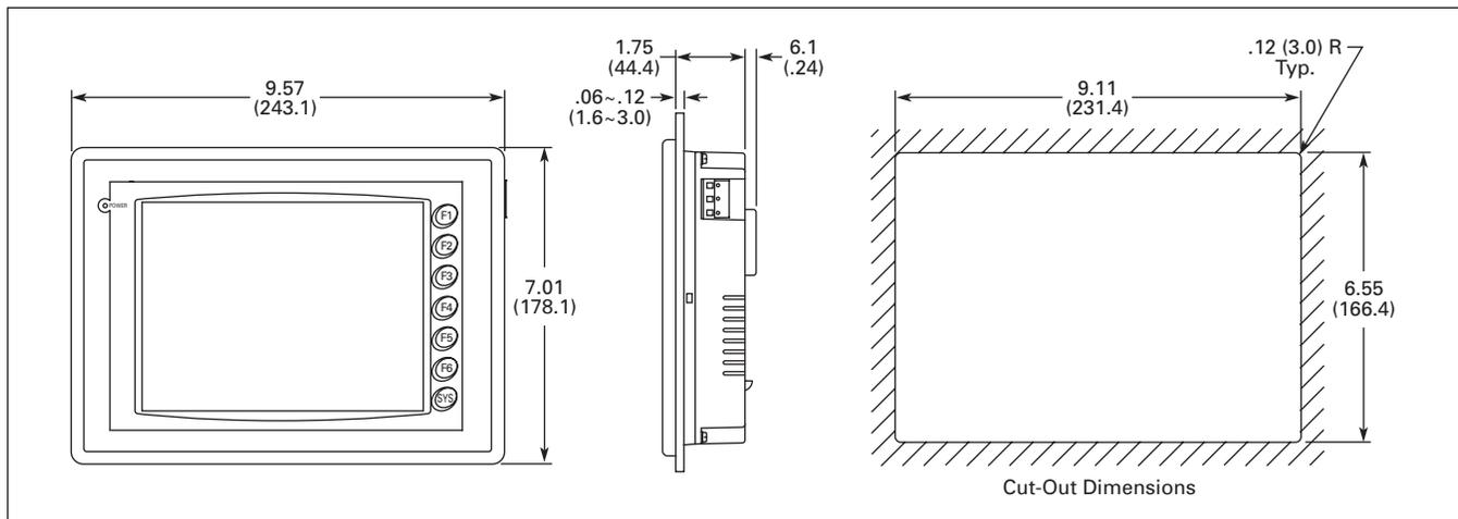
Figure 10. HMI08CE — Approximate Dimensions in Inches (mm)
