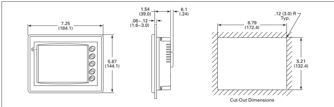
Figure 9. HMI06\_\_ — Approximate Dimensions in Inches (mm)
