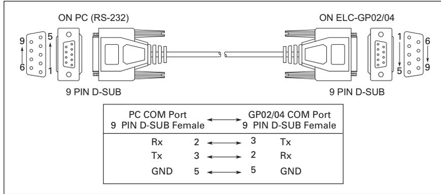
**Figure 2. PC to ELC-GPxx Cable**
