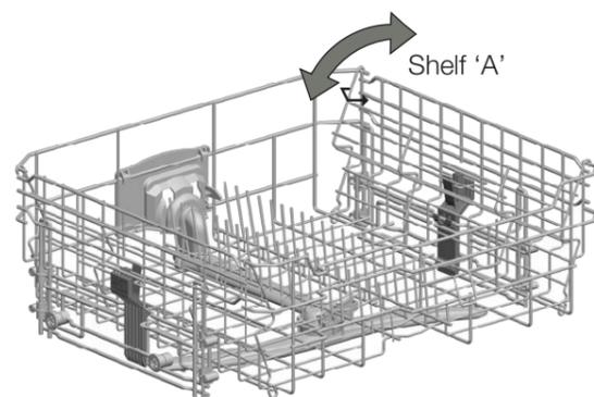
The upper basket height is adjustable. There is a higher and lower position for the upper basket which is used to wash dishes with different heights. You can lift the basket or press the adjustor to the upper and lower position.
