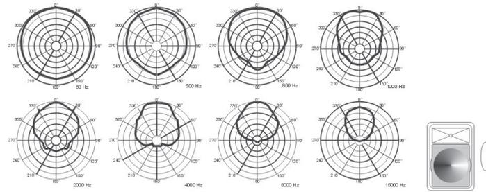
polar response, vertical (60 Hz to 15 KHz)
