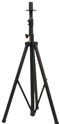
**SPS-1B - Speaker Stands** - American Audio® carries two types of speaker stands that may be used to raise the speakers during use. The SPS-1B is a sturdy aluminum tri-pod and includes a mounting socket bracket for added security. The SPS-1B can raise the speaker to a maximum height of six feet and has a maximum weight capacity of 80 pounds. SPS-1B; weight = 6lbs, pipe diameter - 1 3/8"
