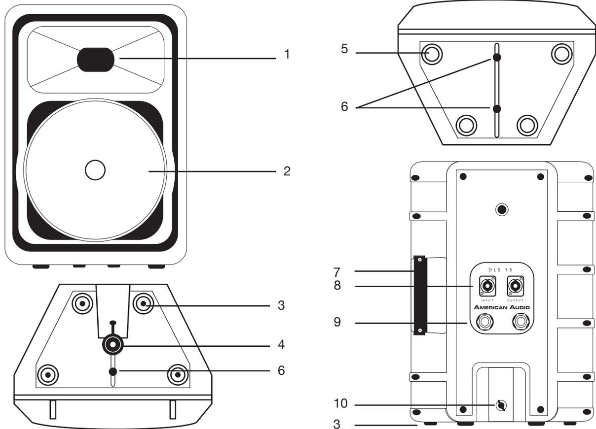
1. **HIGH FREQUENCY TRANSDUCER** – This unit is used to reproduce the high frequency response.
