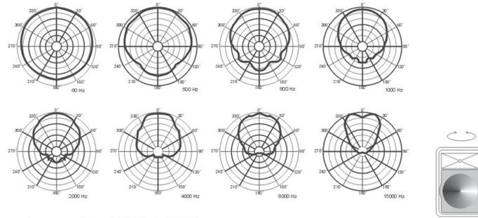
polar response, horizontal (60 Hz to 15 KHz)
