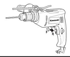
**CAUTION** Do not change the direction of a moving bit. Make sure the bit comes to a complete standstill before moving switch. Changing direction while the bit is moving can cause damage to the drill.
