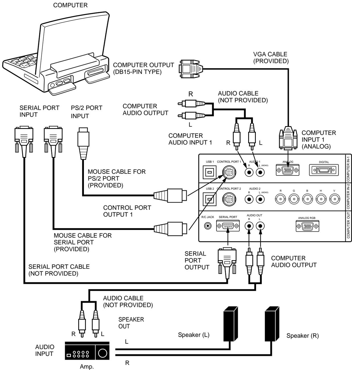
**NOTE:** When connecting the cables, the power cords of both the projector and the external equipment should be disconnected from AC outlet. Turn the projector and peripheral equipment on before the computer is switched on.
