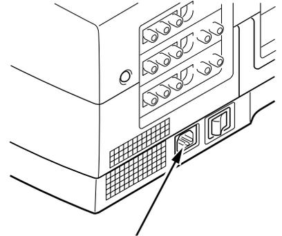
Connect the AC power supply cord (supplied) to the projector. The socket-outlet must be near this equipment and must be easily accessible.
