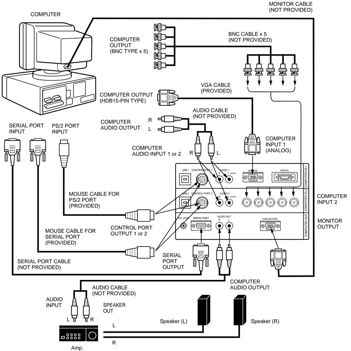
**NOTE:** When connecting the cables, the power cords of both the projector and the external equipment should be disconnected from AC outlet. Turn the projector and peripheral equipment on before the computer is switched on.
