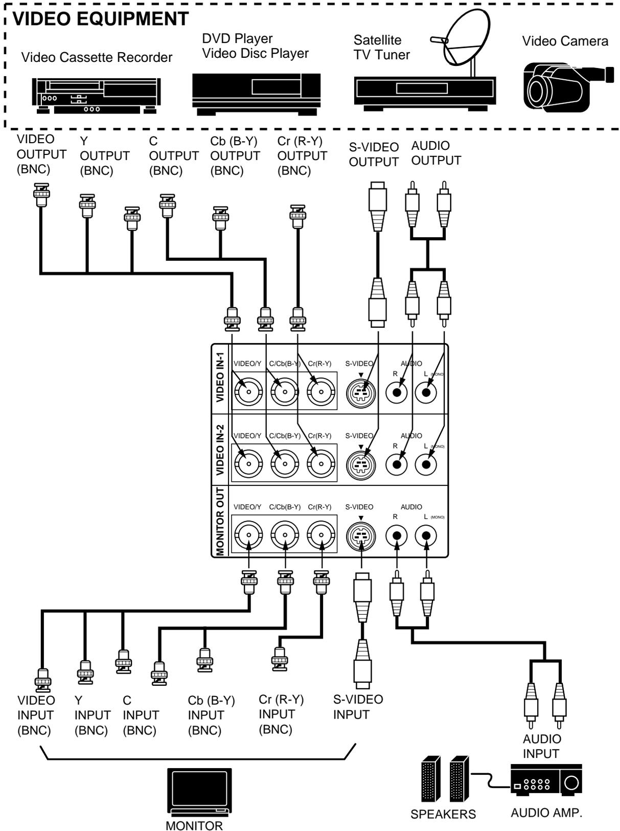
**NOTE:** When connecting the cables, the power cords of both the projector and the external equipment should be disconnected from AC outlet. Turn the projector on before the peripheral equipment is switched on.
