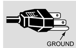
This projector is equipped with a grounding type AC line plug. Should you be unable to insert the plug into the outlet, contact your electrician. Do not defeat the safety purpose of this grounding type plug.
