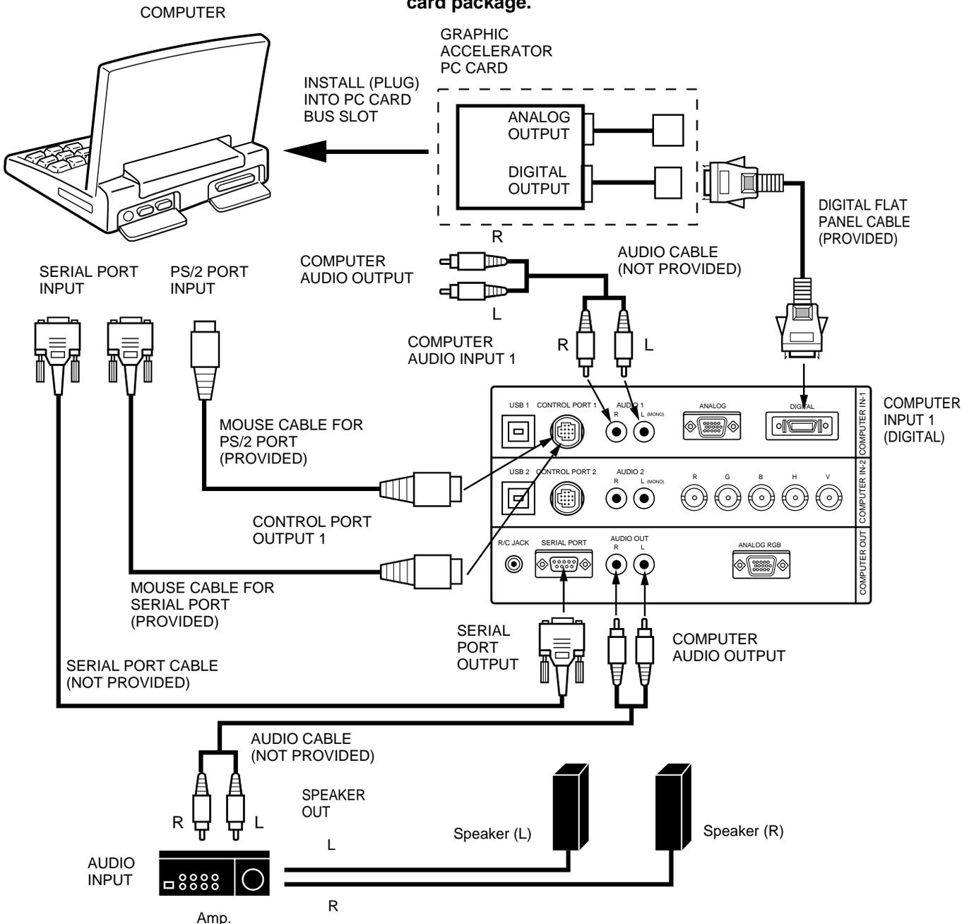
**NOTE:** When connecting the cables, the power cords of both the projector and the external equipment should be disconnected from AC outlet. Turn the projector and peripheral equipment on before the computer is switched on.
