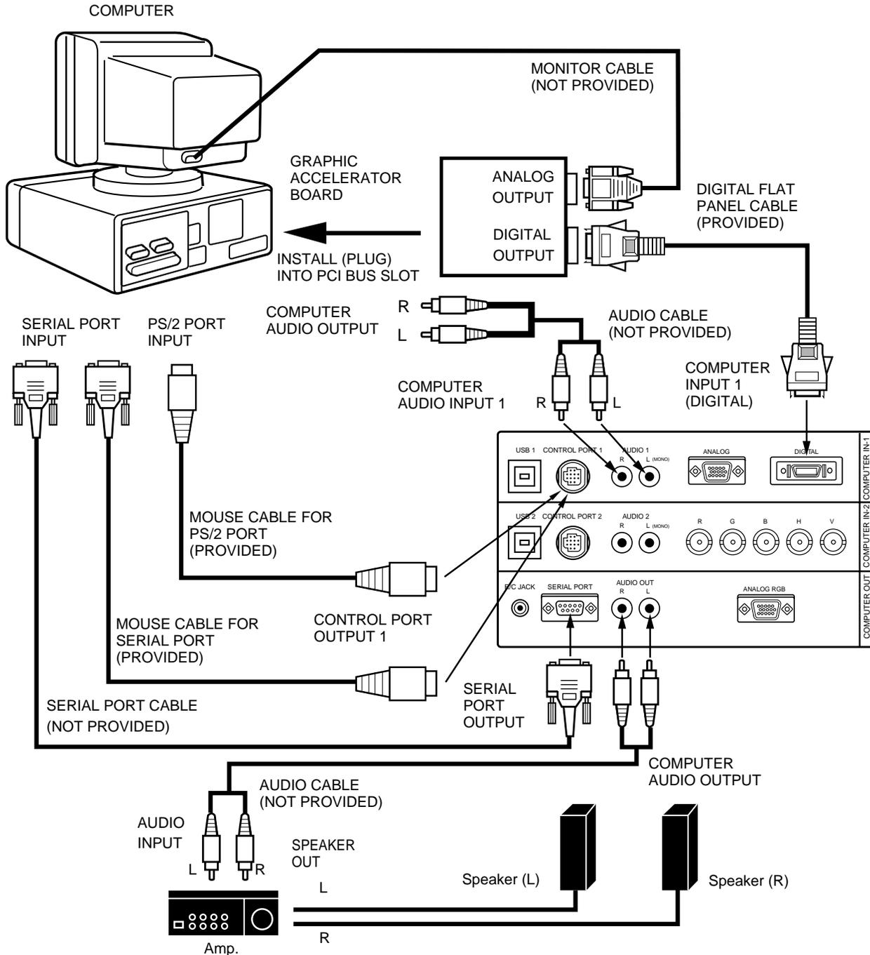
**NOTE:** When connecting the cables, the power cords of both the projector and the external equipment should be disconnected from AC outlet. Turn the projector and peripheral equipment on before the computer is switched on.
