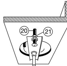
USE SCREWS WITH NUTS TO TIGHTEN UNIT TO COUNTERTOP. WIPE OFF EXCESS CAULKING.
