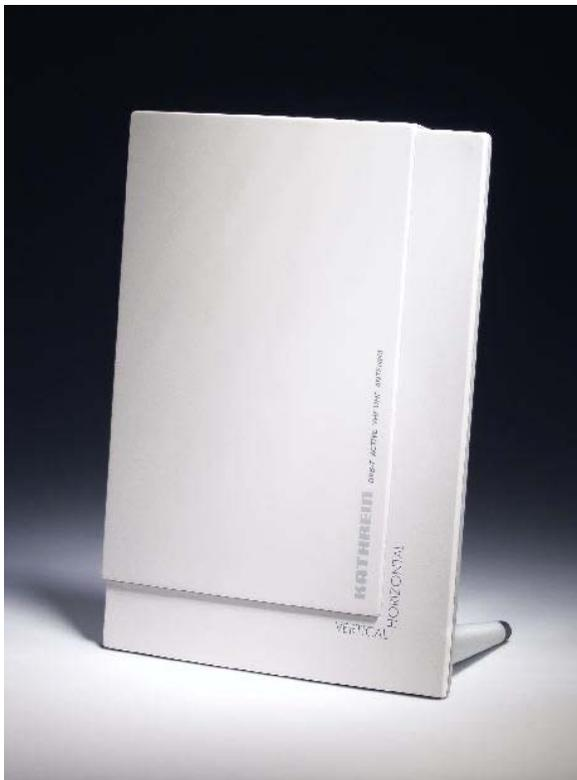
The antenna's reception range is 174-230 MHz in the VHF band and 470-862 MHz in the UHF band. As the BZD 30 is virtually omni-directional, no special alignment is required.
