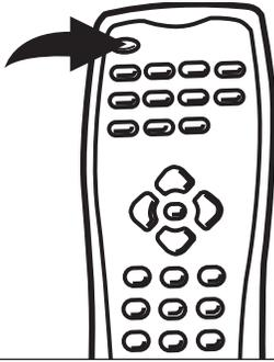
Press the POWER button to turn on the TV; the POWER indicator will light green.
