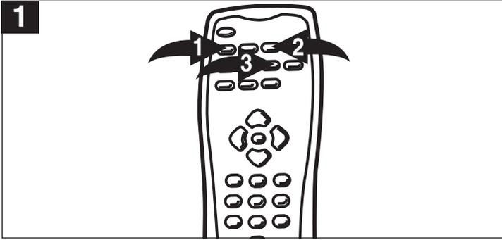
Press the MUTE button ❶ to turn off the sound. The TV's sound will be silenced and "MUTE" will appear on the screen. The sound can be turned back on by pressing this button again or the VOLUME Up ❷ or Down ❸ button.
