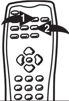
Adjust the volume level by pressing the VOLUME Up ❶ or Down ❷ button. The volume level will be indicated on the screen by green bands and a green numerical display between 0 and 24 where 0 is the lowest setting and 24 is the loudest.
