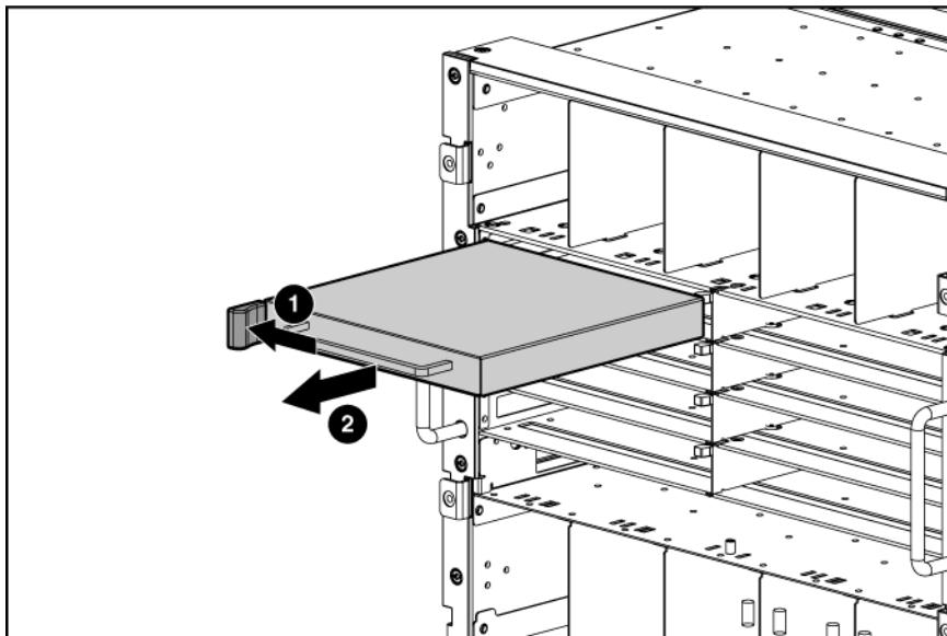
2. Open the handle on the pass-thru module.
