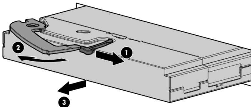
3. Slide the new module fully into the interconnect bay. For more installation information, see "Installing the module (on page 9)."
