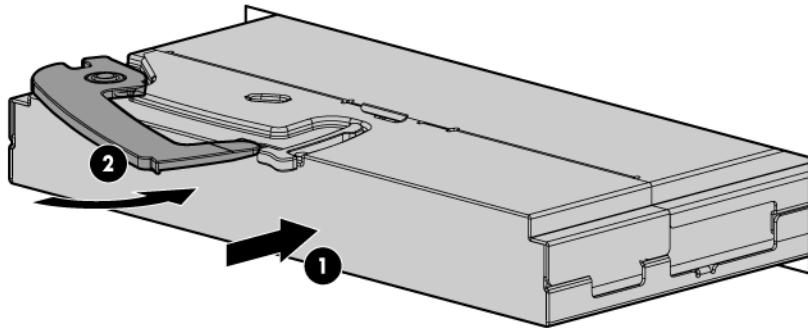
Complete installation is indicated by a green Health LED. If the Health LED is amber or power is not applied to the module, see the HP BladeSystem Enclosure Setup and Installation Guide for troubleshooting information.
