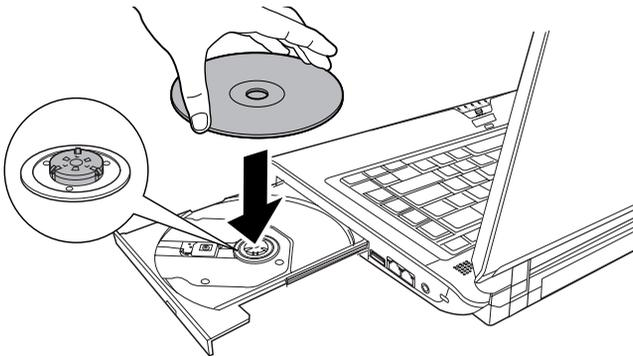
*Inserting a disc*
