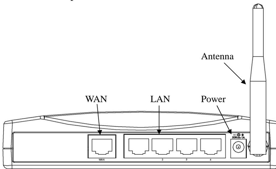
Figure 2 – X-Micro WLAN 11b Broadband Router Rear Panel
