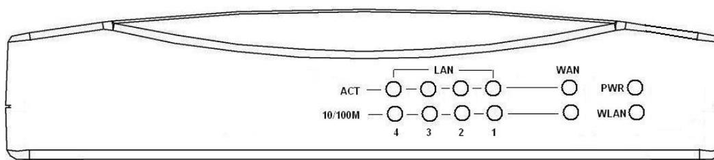
Figure 1 – X-Micro WLAN 11b Broadband Router Front Panel
