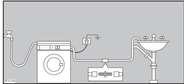
**For a correct functioning of the machine the drain hose must remain hooked on the proper support piece situated on the top part of the back side of the appliance.**
