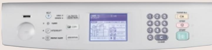
◀ The easy-to-use touch-screen LCD display guides users through features and options with simple prompts and a convenient "HELP" key. A Graphic Service Guidance System provides step-by-step instructions for replacing toner, removing misfeeds, and more.
