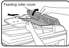
Open the feeding roller cover and pull the original gently to the left and out from the document feeder tray. Close the feeding roller cover.
