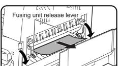
Carefully remove the misfed paper. Lower the fusing unit release levers to allow easier removal. Return the release levers to their operating positions.
