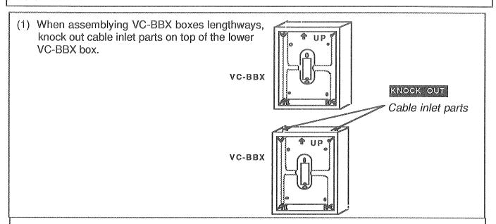
(2) Be careful that cable should be run so as not to be pinched by the illumination plate.
