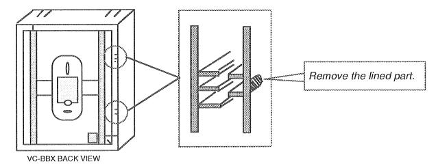
(3) Assemble two VC-BBX boxes with two connecting blocks.
