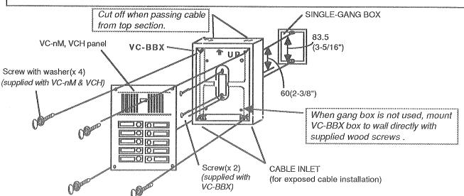
As shown, VC-BBX may be mounted on single-gang box or to wall directly. Two cable inlets are provided at the bottom on VC-BBX, or may be introduced from top of VC-BBX, by removing either of two inlet parts by a knife.
