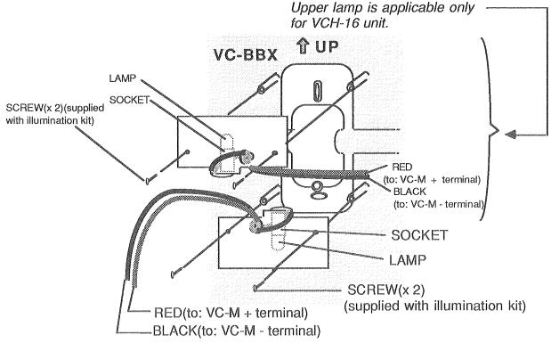
As shown, attach the back illumination lamp at the lower studs for VC-nM and VCH-8 units.
