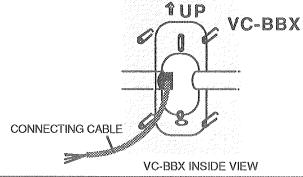
Dimensions: H: 264 x W: 190 x D: 52(mm)(10-3/8" x 7-1/2" x 2-1/16") 59mm(2-5/16") deep with VC-M panel mounted on VC-BBX.
